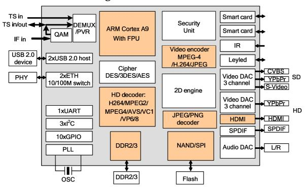
With the advanced ARM Cortex A9 processor, Hi3716M V300 provides high-speed processing capability, which meets the requirements of complex applications. As Hi3716M V300 has two built-in Ethernet ports and two USB ports, it supports flexible connection solutions. Hi3716M V300 also supports high-definition video decoding in various formats (including MPEG2, H.264, and AVS, VC-1 AP, VP6/VP8) to meet multi-media playing requirements.
